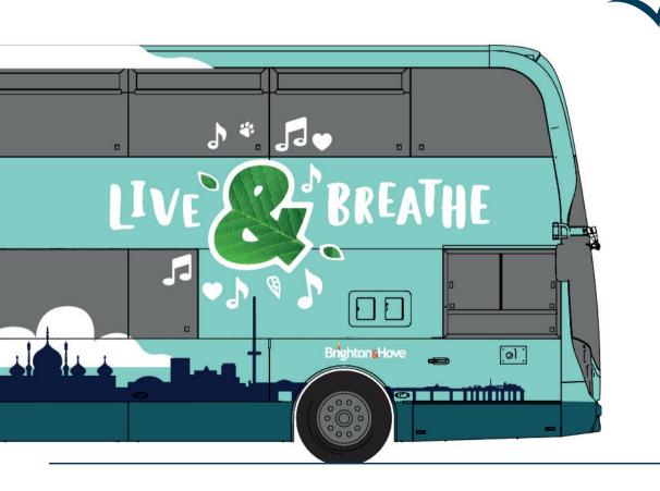
54 ADL E400ER hybrid electric buses with geo-fenced zero emission electric only operation through the city's Low Emission Zone delivering 244,000 miles of zero emission bus travel every year over 3 million passenger journeys.
